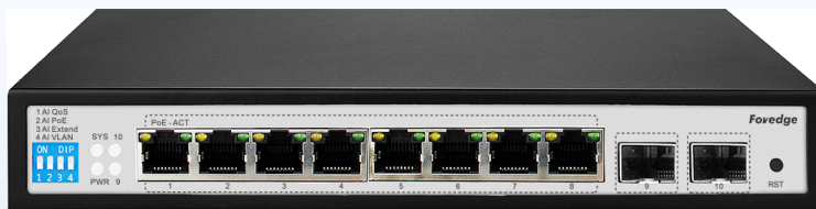
Front panel — 8 gigabit PoE ports, 2 SFP fibre uplinks, status LEDs and the AI mode button
