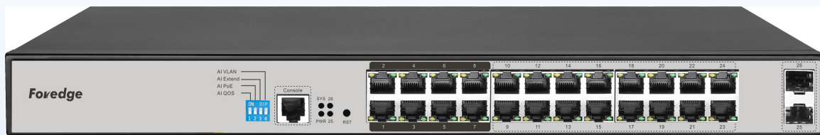
Front panel — 24 gigabit PoE ports, 2 SFP fibre uplinks, console port and the AI mode button
